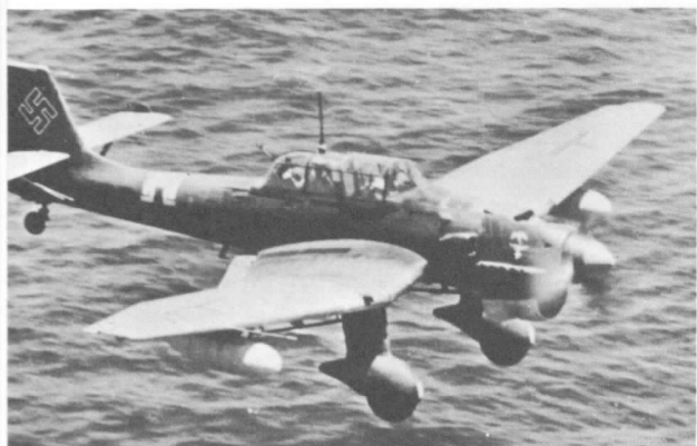
Below: Ju 87D in Russia, summer 1943. Note that the aircraft is painted in conventional splinter camouflage all over—unusual for this type of unit—and that the badge of 7 Staffel, Stukageschwader 1 is marked on the cowlings. The rims of the machine gun ports in the wing leading edges are painted yellow.
