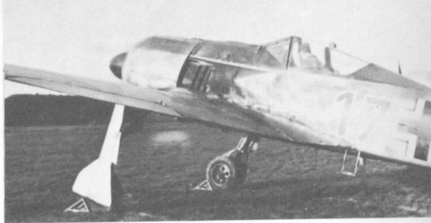
Above: Standard camouflage on an Fw 190A; note the extended flash of black paint over the exhaust area, peculiar to this type of fighter. (U.S. National Archives).
