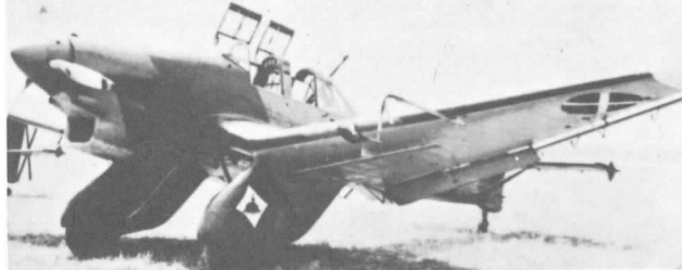
One of the Junkers Ju 87A Stukas which served with the Condor Legion; the camouflage is standard Luftwaffe segment scheme, with Spanish Nationalist markings. The undercarriage spats bear a unit badge, and note the yellow and red striping of the propeller blade tips. (Obert).
